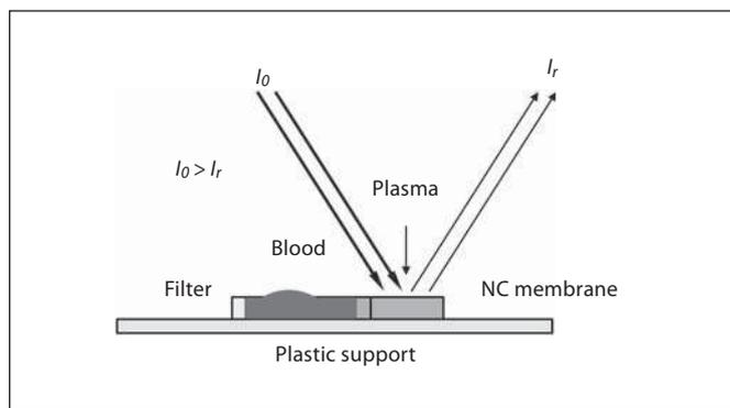
**Fig. 1.** Schematic diagram of the Bilistick system and its functionality. After 25- $\mu$ l blood loading onto the filter, the plasma passes the capillary tube to the NC membrane. When the strip is inserted in the reader, the intensity of reflected light  $I_r$  is measured by the device to calculate the bilirubin concentration.
